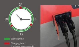
Lithium battery forklift truck is equipped with double gun charging as standard, which greatly reduces the charging time. Lithium batteries have high-density capability and can be used and charged at any time to realize efficient and continuous operation all day long.
